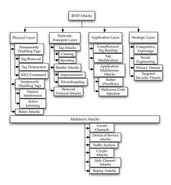
Fig. 2. Classification of RFID attacks.
