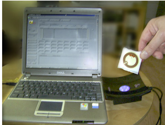
Fig. 2. The world's first virally infected RFID tag.
