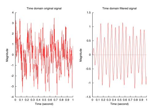
Figure 24.10: The original and filtered signals in the time domain.
