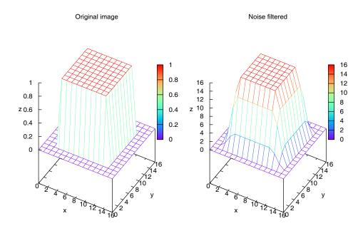
Figure 24.12: The original image and filtered one using function **filter**2().
