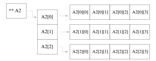
Figure 14.2: Dynamic allocation of two-dimensional arrays (method 2).
