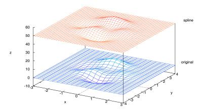
Figure 24.4: The result from two-dimensional interpolation function **interp2**().
