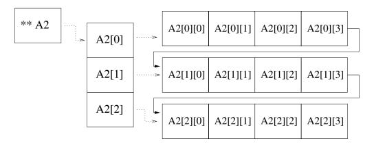
Figure 14.1: Dynamic allocation of two-dimensional arrays (method 1).
