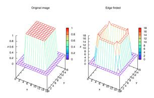
Figure 24.9: The result from two-dimensional convolution function **conv**2().
