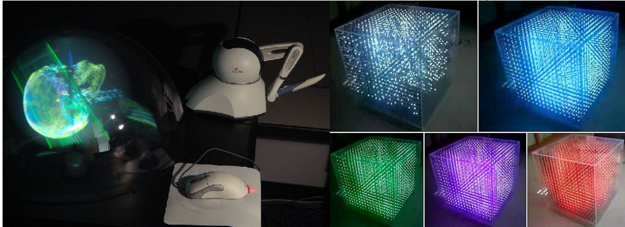
Figure 1. Photograph of the Perspecta volumetric display courtesy Actuality Systems, Inc. and RGB LED cube from Seekway
