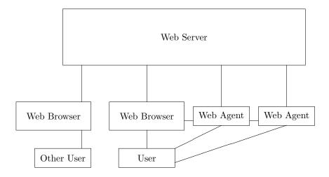
Fig. 6.8 Configuration of 2D-client-multiple-agent
