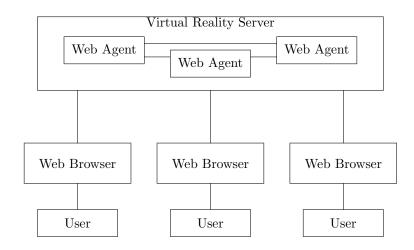
Fig. 6.2 Configuration of 3D-server-multiple-agent
