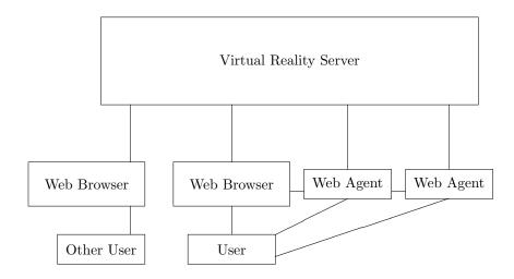
Fig. 6.4 Configuration of 3D-client-multiple-agent
