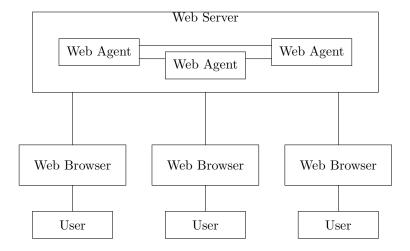
Fig. 6.5 Configuration of 2D-server-multiple-agent
