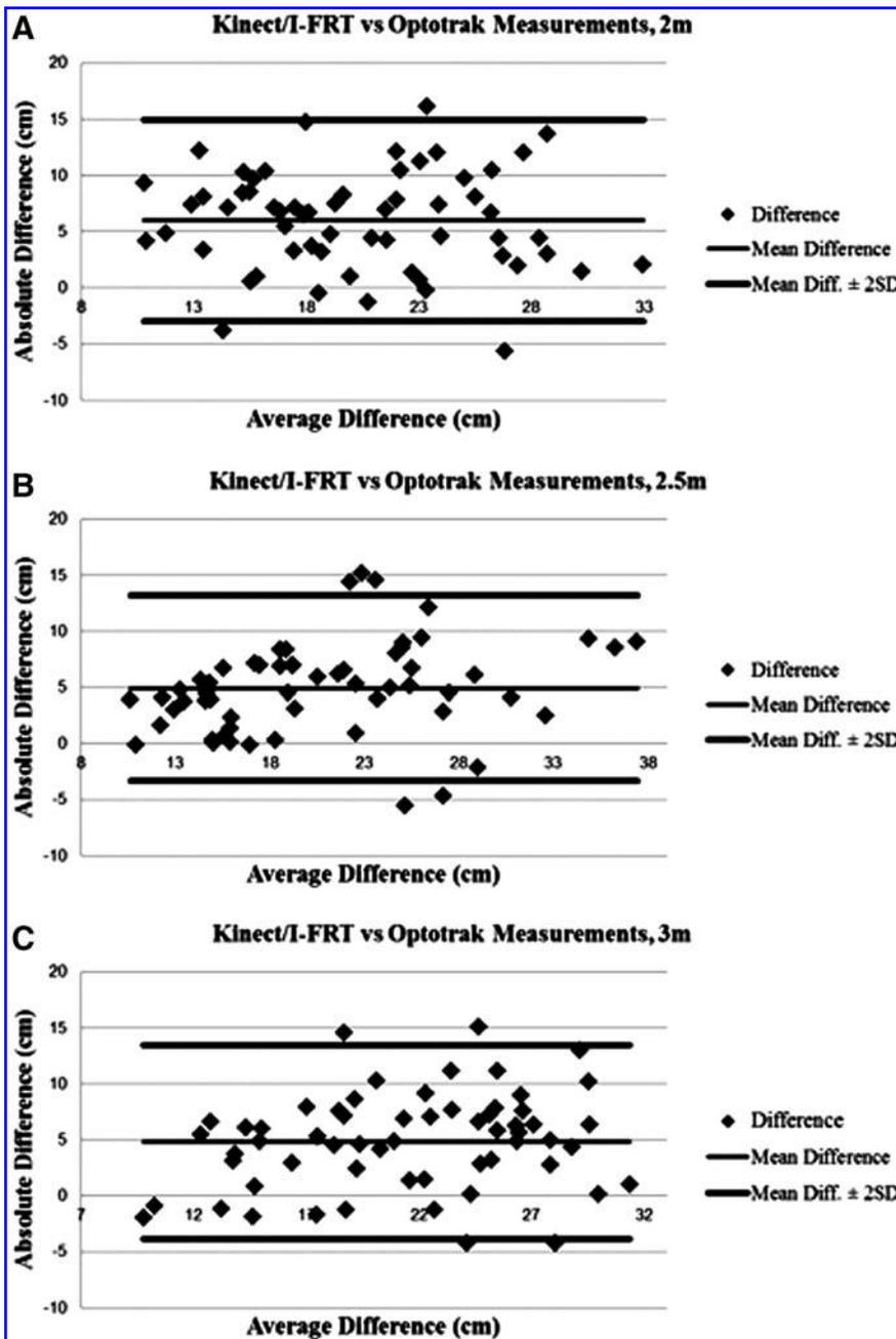
**FIG. 4.** Bland–Altman plots showing the distribution of absolute difference between the measures of the Interactive Functional Reach Test (I-FRT) and the Optotrak systems around the mean difference: (A) 2 m, (B) 2.5 m, and (C) 3 m. SD, standard deviation.
