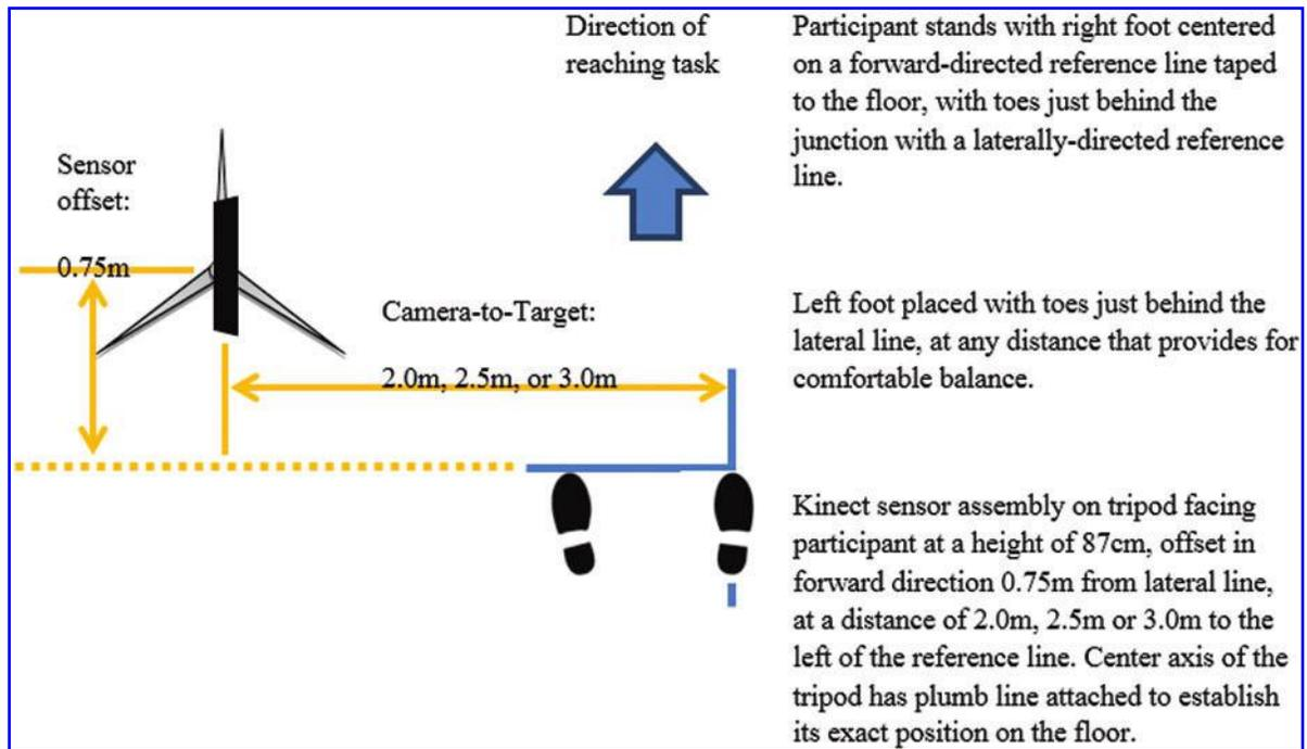
FIG. 2. The experimental set-up. Color graphics available at [www.liebertonline.com/g4h](http://www.liebertonline.com/g4h)
