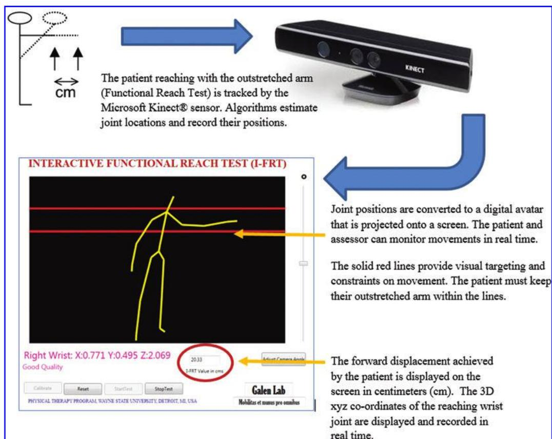
**FIG. 1.** Schematic showing the set-up and implementation of the Interactive Functional Reach Test. 3D, three-dimensional. Color graphics available at [www.liebertonline.com/g4h](http://www.liebertonline.com/g4h)
