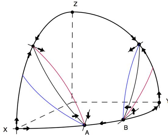
**FIGURE 4.5** Schematic figure of the behaviour of the flow around the equilibrium points, obtained by classifiable equilibrium points and nullclines. All trajectories move towards  $A$ , hence being the only stable equilibrium point.
