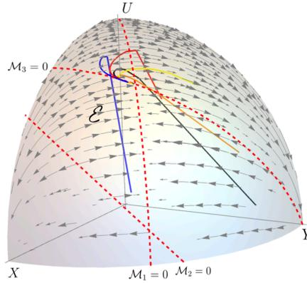
**FIGURE 6.9** In the system where  $V_1$  is the smallest growth rate all the trajectories converge to some equilibrium point where  $Q_1 = Q_2 = Q_3 = V_1$ .
