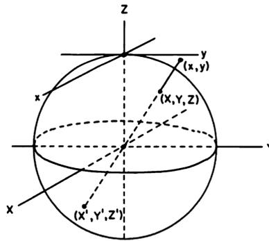
**FIGURE P.2** Projection of the  $(x, y)$ -plane onto the surface of the unit sphere in the  $(X, Y, Z)$ -space.
