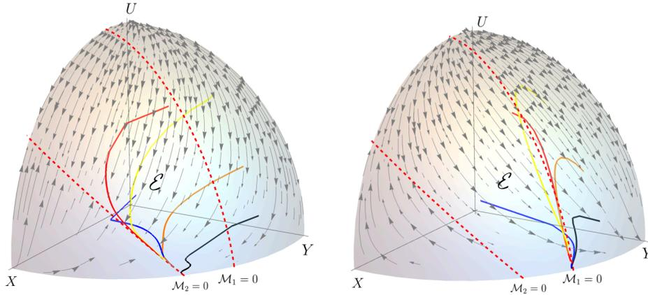
**FIGURE 6.3** The left figure shows the stream plot on the equator and some trajectories that come from inside the ball, when  $V_1 > V_2 > V_3$ ; the right figure shows the case  $V_2 > V_3 > V_1$ . The figures are made for relatively small time  $t$  to improve the accuracy of the shown trajectories, at the expense of the long-term behaviour, since it converges slowly towards the equilibrium point when it is near  $\mathcal{M}_i = 0$  for some  $i$ .
