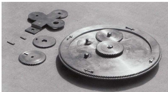
Fig. 17. The epicyclic gearing showing the pin and slot coupling between the wheels on the K-axle [20]
