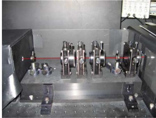
Figure 5-20: Light cleaning stage. The light goes from right to left, and its path is shown in red. The first holder contains the collecting lens L4, followed by a diaphragm (D2) and then by the set L5-S2-L6 of lens, pinhole and lens. The diaphragm D3 is the last components shown. The additional diaphragm D<sub>2</sub> is placed to facilitate alignment, but it does not play any role in the signal collection.
