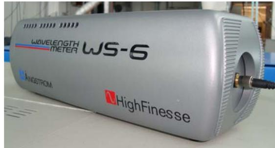
Figure 3-12: Photograph of the Fizeau spectrometer with an optical fiber input and an USB computer interface.
