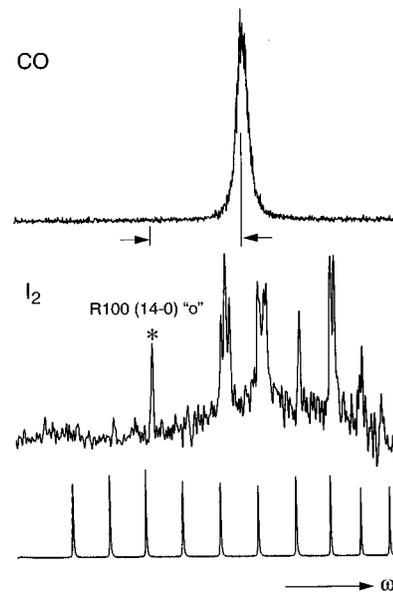
Fig. 5. Spectrum of the  $Q(1)$  line of the  $L^1\Pi-X^1\Sigma^+(0,0)$  band of CO recorded simultaneously with a Doppler-free  $\text{I}_2$  spectrum and an etalon spectrum. This spectrum was recorded from a pure CO beam, without use of the EOM for chirp compensation. The absolute frequency of the  $Q(1)$  line is calibrated with respect to the  $\text{I}_2$  line marked by an asterisk at  $17\,211.96456(20)$   $\text{cm}^{-1}$ .
