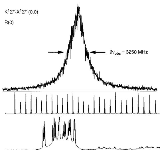
Fig. 2. Spectrum of the  $R(0)$  transition of the  $K^1\Sigma^+ - X^1\Sigma^+(0,0)$  band of CO recorded by 1XUV + 1UV photoionization at  $\lambda = 97.03$  nm. Etalon markers (in the middle panel) and an  $I_2$  saturation spectrum (lower panel) are on-line recorded with the output of the cw ring dye laser.
