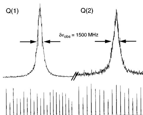
Fig. 3. Spectrum of separately recorded  $Q(1)$  and  $Q(2)$  lines of the  $W^1\Pi - X^1\Sigma^+(0,0)$  band of CO recorded by 1XUV + 1UV photoionization at  $\lambda = 97.27$  nm. Also shown are transmission fringes of a stabilized etalon used for the determination of the linewidths.
