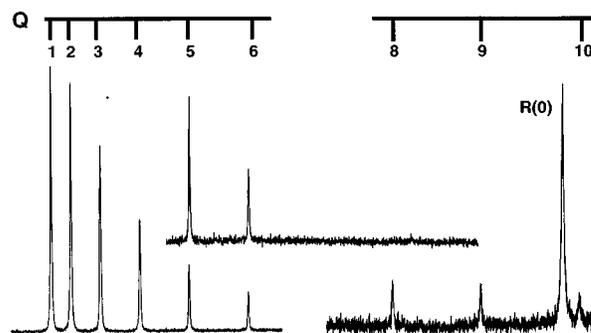
Fig. 4. Excitation spectrum of the  $L^1\Pi - X^1\Sigma^+(0,0)$  band of CO in the bandhead region of the  $Q$  branch by 1XUV + 1UV photoionization at  $\lambda = 96.83$  nm, recorded in three separate overlapping scans. Note that the  $Q(7)$  line is missing.
