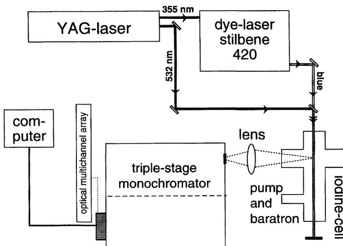
FIGURE 2 Schematic representation of the experimental setup.
