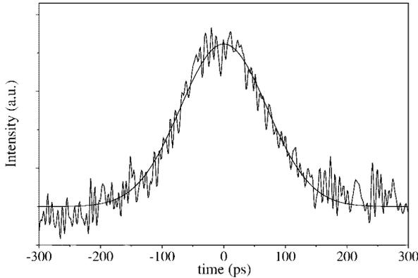
Fig. 4. Streak camera trace of the secondary compressed pulse in water. The measured pulse duration (FWHM) is 160(10) ps much shorter than the phonon lifetime  $\tau_p$ .
