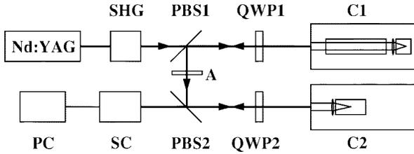
Fig. 3. Experimental setup of double compressor. SHG: second-harmonic generation stage; PBS: polarizing beam splitter; QWP: quarter-wave plate; A: attenuator; C: Brillouin compressor; SC: streak camera; PC: personal computer.
