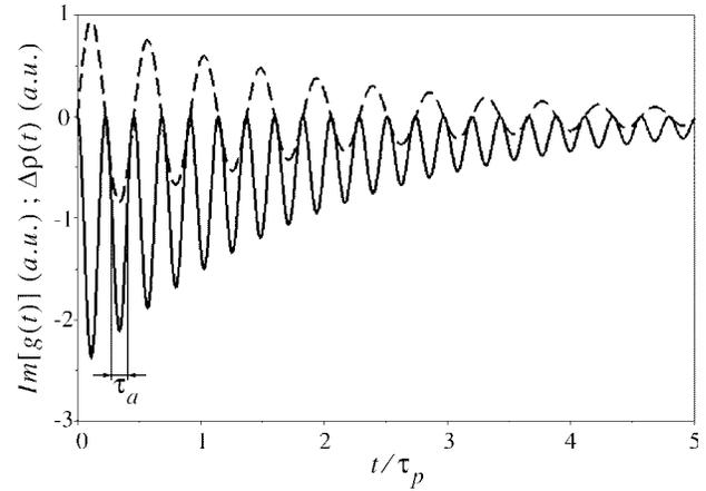
Fig. 1. Imaginary part of the gain function  $g(t)$  (solid line) and the acoustic field  $\Delta\rho(t)$  (dashed line) generated by a short  $\delta$ -like pulse in water for  $\lambda = 532$  nm. Note that the ratio  $\tau_p/\tau_a$  is a material property.
