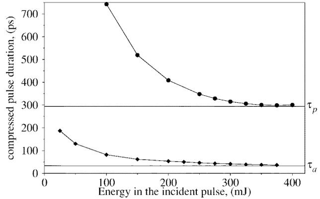
Fig. 2. Calculated compressed pulse duration *versus* energy in the incident pulse for a 10-mm beam diameter. Circles: input pulse of 5 ns; diamonds: input pulse of 600-ps duration.
