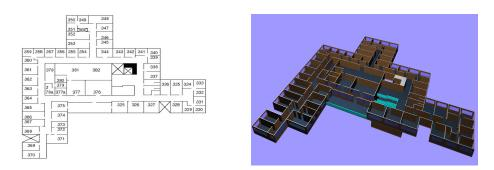
On the left is the 2D map of the third floor of CWI, on the right the model generated from it.
